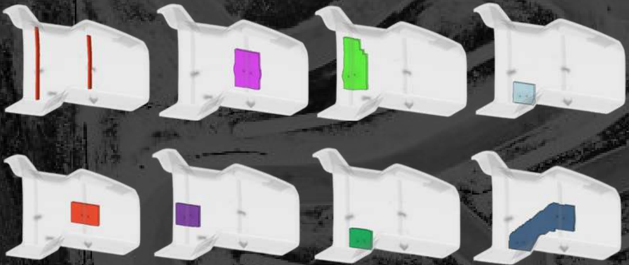
Stiffeners and Reinforcement Geometry and Placement for Front Suspension
